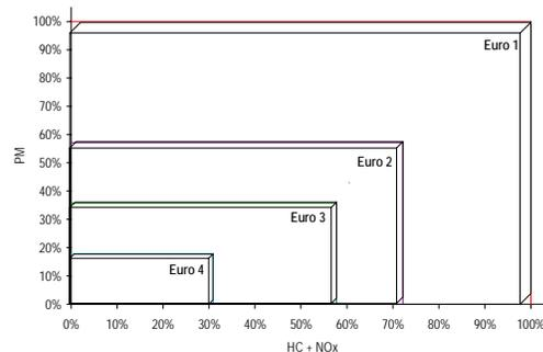
Figure 3. Plot showing the relative reduction in emissions limits of the European emissions legislation for diesel vehicles
